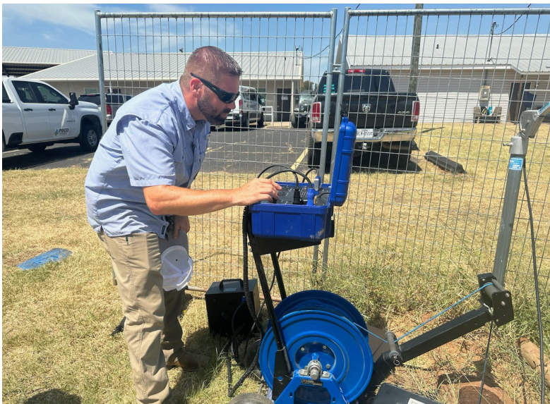
Field Operations Coordinator, Michael Heath, operating a down hole camera during a field collaboration with Upper Trinity GCD.
