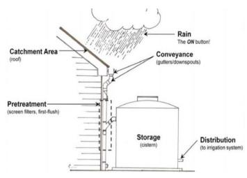
A domestic rainwater harvesting system comprises six basic components:
